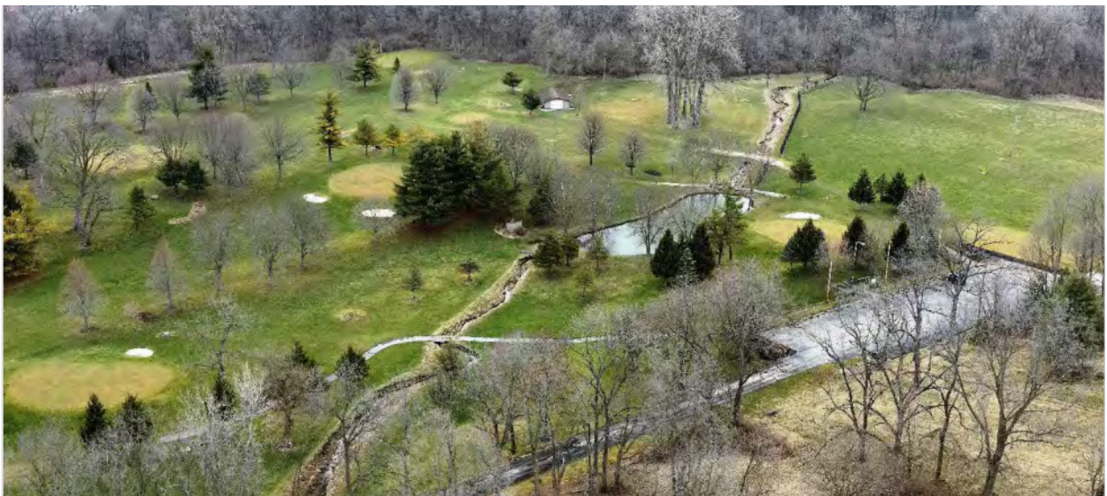
Current conditions prior to the stream and wetland restoration. The tributary exhibits low sinuosity.
